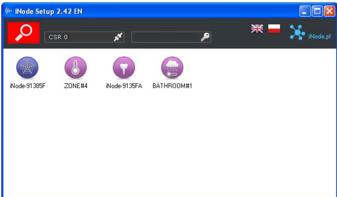
To configure **iNode Serial Transceiver UART** device you should double click on its icon. Application connects with this device and reads its settings:
