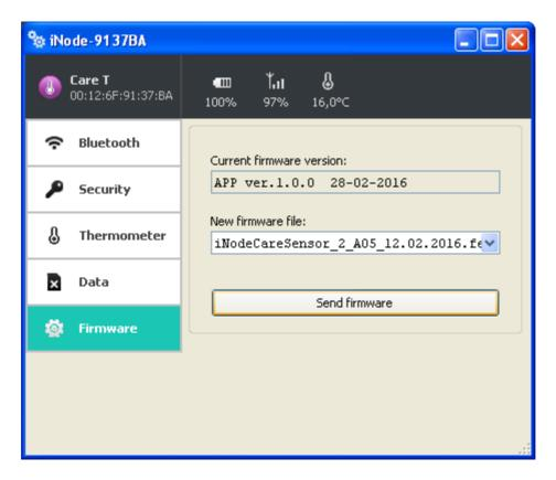
**Current firmware version** field shows the version and creation date of the firmware in the device.
