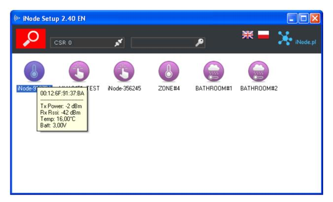
To configure **iNode Care Sensor T** device you should double click on its icon. Application connects with this device and reads its settings:
