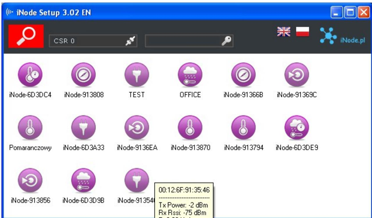
To configure **iNode Care Sensor PT** device you should double click on its icon. Application connects with this device and reads its settings:
