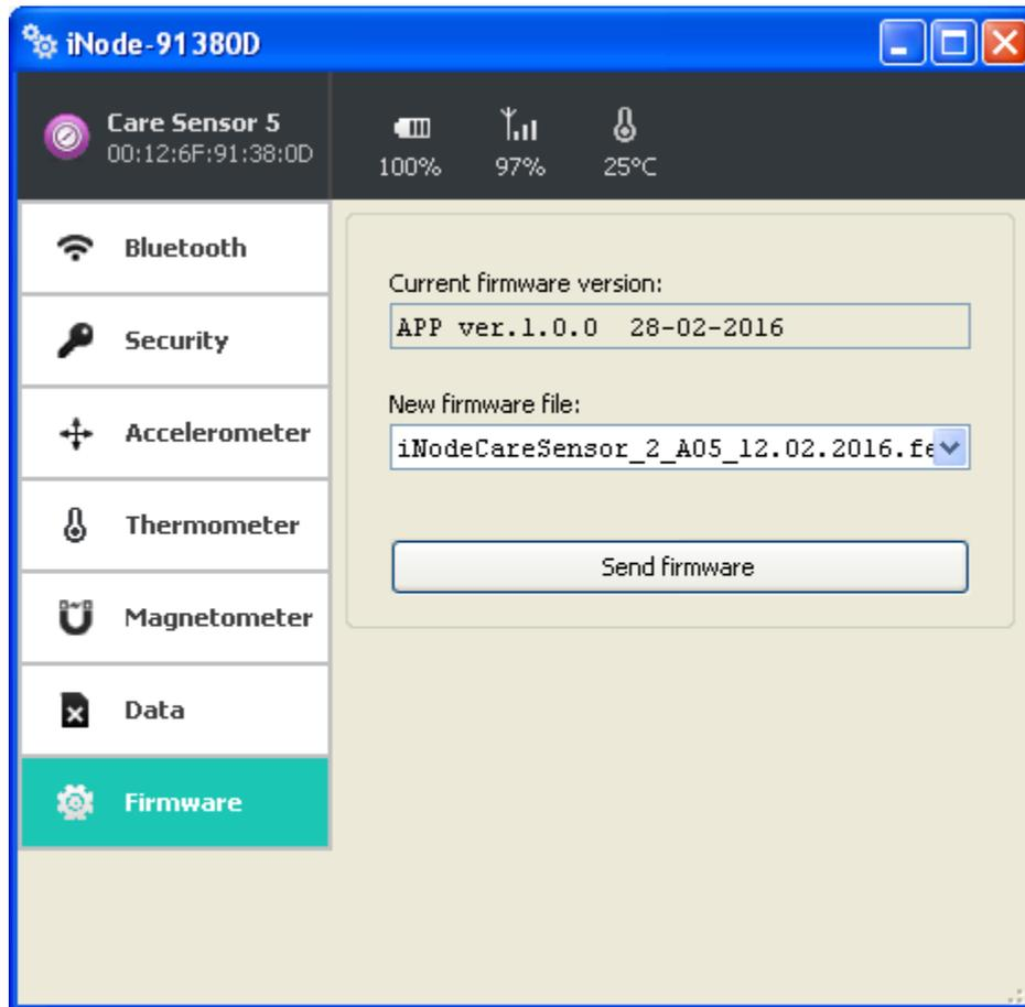
**Current firmware version** field shows the version and creation date of the firmware in the device.
