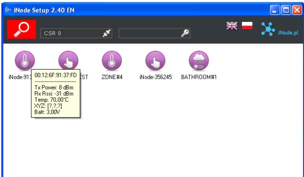
To configure **iNode Care Sensor #2** device you should double click on its icon. Application connects with this device and reads its settings:
